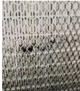
Figure 7: Rupture in the pleats in a panel pleated filter
