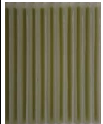
Figure 3: A close-up of a few minipleats separated by hot melt
