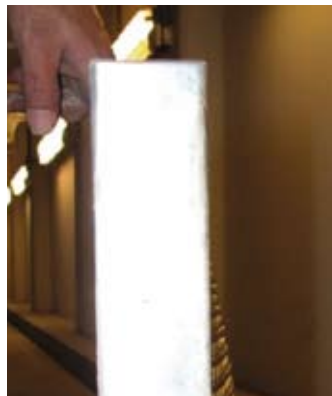
Figure 8: Deformation of the entire filter pleated panel
