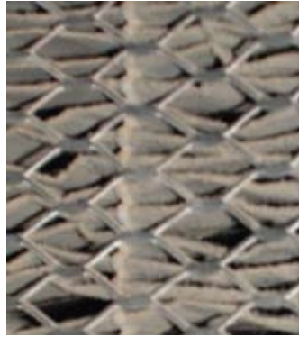
Figure 6: Pleat distortion after being subjected to high flow rates
