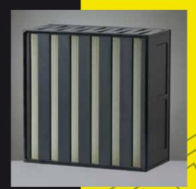
EMW® filter boxes provide extremely high filter surface areas ranging up to 40m². The filter media are bonded to the electrically dissipative frame by a cast airtight joint. The reliable full-perimeter bond prevents leakage even at highest flow rates. In addition the IECEx filter boxes are available with a continuous foamed-in-place seal located on the air inlet or outlet side as desired.
