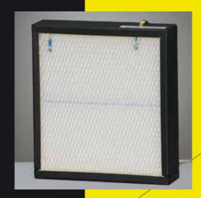
IECEx minipleat panel filters are supplied with integrated earthing lugs. These pleated filter media are offered in plastic frames in all common dimensions. The filter media are high quality, wet-laid glass-fibre materials and sealed in the frame by a cast airtight joint.
