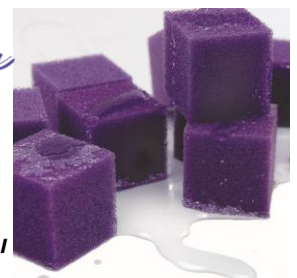
Poret®aqua following 2 years' field service in concrete MBBR.
