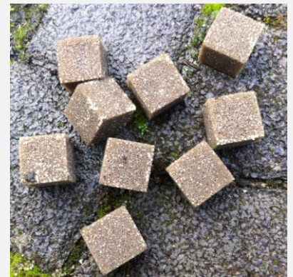
Poret®aqua following 2 years' field service in concrete MBBR.
