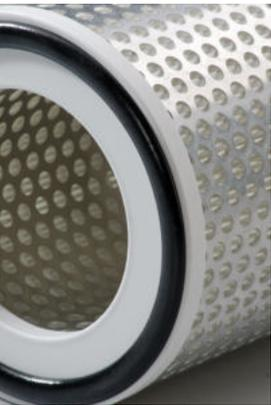
EMW® cartridge filters are available in ISO 16890 (formerly EN 779) Filter Classes and EN 1822 Filter Classes E10-H14. Their multiple filter medium is securely mounted on the plastic frame with a cast airtight joint. A continuous foamed-in-place seal over the joint further ensures airtightness. A perforated metal guard is available as an option for additional stability under high aerodynamic stress.
