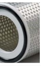
EMW® cartridge filters are available in EN 779 Filter Classes M6-F9 and EN 1822 Filter Classes E10-H14. Their minipleat filter medium is securely mounted on the plastic frame with a cast airtight joint. A continuous foamed-in-place seal over the joint further ensures airtightness. A perforated metal guard is available as an option for additional stability under high aerodynamic stress.
